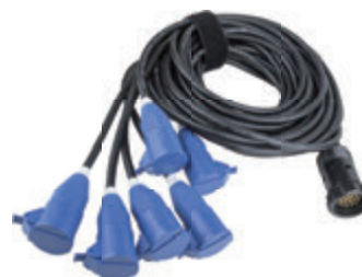
Cable: H07RN-F 3x1.5mm 2 or 2.5mm 2 Connector: 19pin (input) / Schuko 13A (output)
